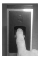
Read the Master card 5 times in the Lock,Can hear two short "Di Di",The delete is successful.
