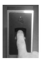
After reset, Use a new card to swipe the lock, After 2 short sounds "Di Di", The Master card is working
